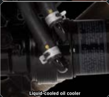
Liquid-cooled oil cooler
