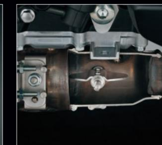
SET valve cutaway
