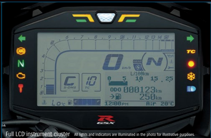
Full LCD instrument cluster All lights and indicators are illuminated in the photo for illustrative purposes.
