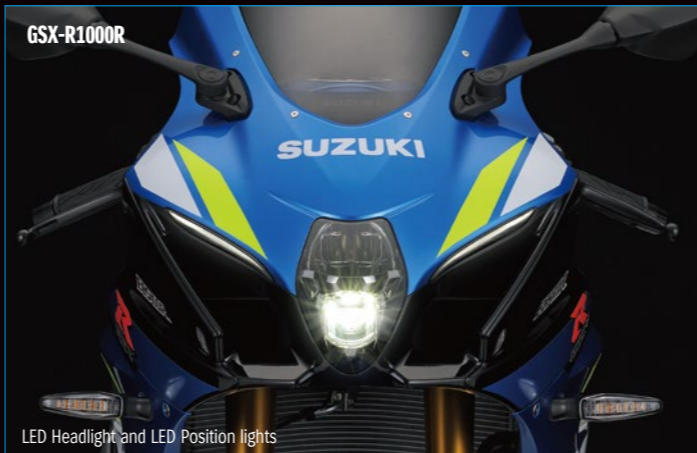
LED Headlight and LED Position lights
